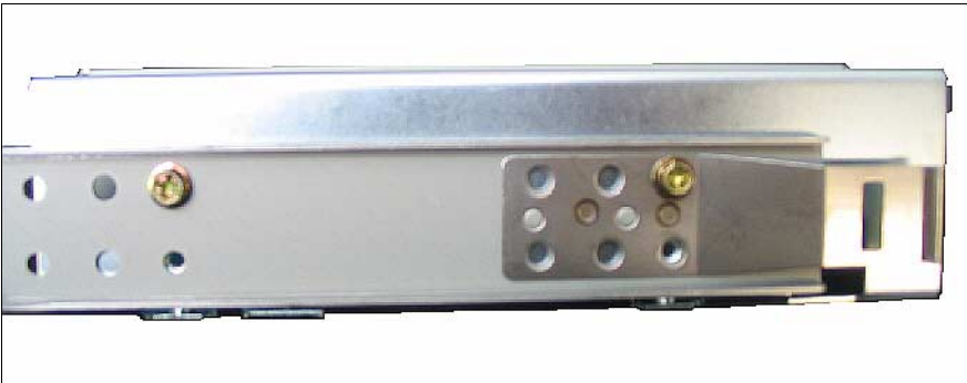
Figure 20: Attaching the EasyClick rails - magnetic tape drive DDS Gen5
